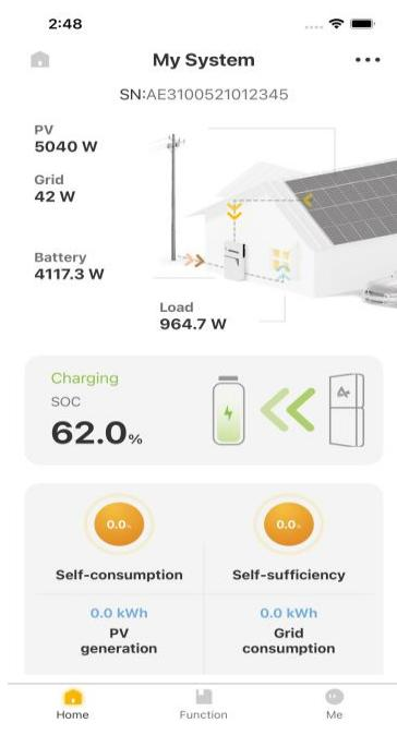
The relative value should be as follows: Load = PV  $\pm$  GRID – Battery
