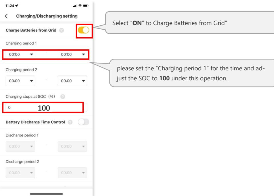
Select "ON" to Charge Batteries from Grid"
