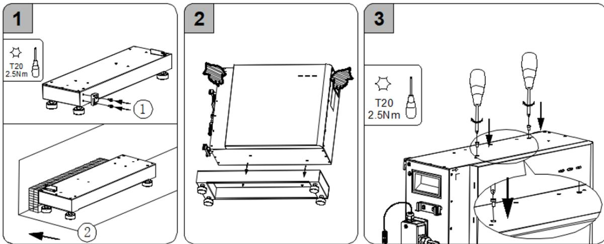
For SMILE-G3-BAT-4.0S, installers need to mount two limit blocks to the top of the batteries for stacking positioning of upper battery.
