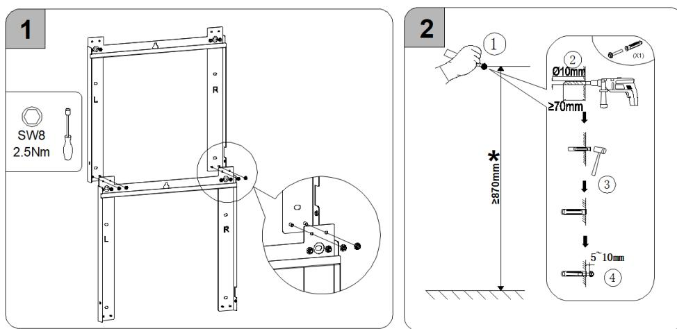
\*This recommended value "870mm" is for wall bracket location of the second battery seeing from the bottom up. Depends on the number of expansion batteries mounted later.
