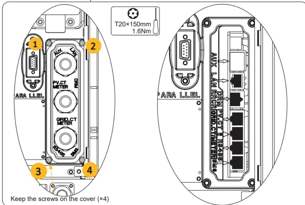
2. Pass the communication cables through the cable glands of the COM connection cover. Do not tighten the strain relief nuts of the cable glands yet.
