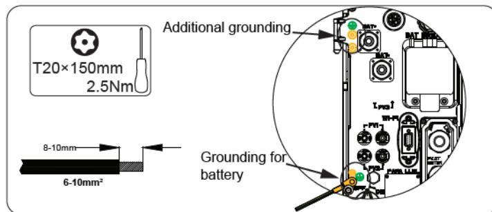
Grounding connection with series battery
