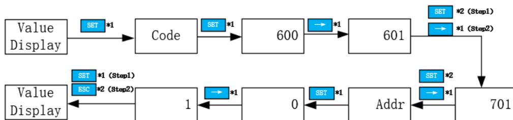
When the meter is used as PV meter, please follow the steps below to complete the address setting.
