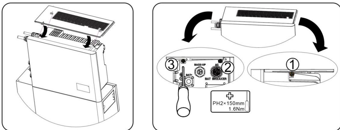
b. Mount right cover of the inverter, align the hooks on the side of the right cover with the slots on the front cover side, and downwards insert the right cover along the edge of the inverter front cover.
