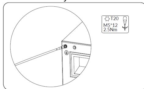
Grounding connection with parallel battery
