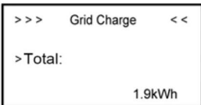
Grid Charge interface displays total battery energy charging from the grid.
